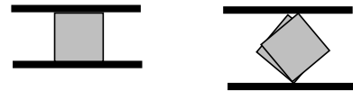
Figure 5: The grasp configuration on the left is stable; those on the right are not.
