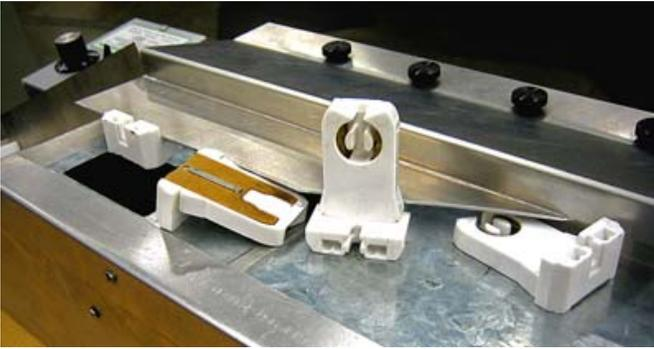
Fig. 2. A side view of the blade feeding the fluorescent fixture mount. Normally, parts fall off the side of the track as illustrated in Fig. 1, but for practical reasons we mimicked this mechanism with the (black) cut-out in the track. The leftmost orientation is fed by the blade, the rightmost orientation will after reorientation end up as the leftmost orientation and thus will also survive the blade, while the middle two orientations will be rejected.
