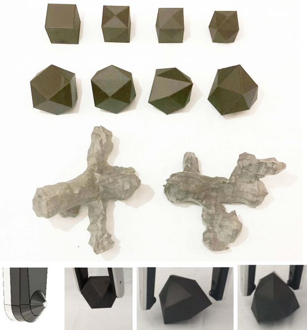
Fig. 5: Top: 3D printed objects with nylon plastic material. We use cubes and cuboctahedrons with \varphi = 0, 10, 15, 26 and adversarial intersected cylinder objects generated by the CEM + GAN algorithm. Bottom (left to right): Gripper design with metal ball bearings to simulate point contacts, successful grasp of the original cuboctahedron, attempted grasp on adversarial cuboctahedron ( \varphi = 26 ), failure on adversarial cuboctahedron ( \varphi = 26 ) in which the object rolls forward after slipping out of the gripper.
