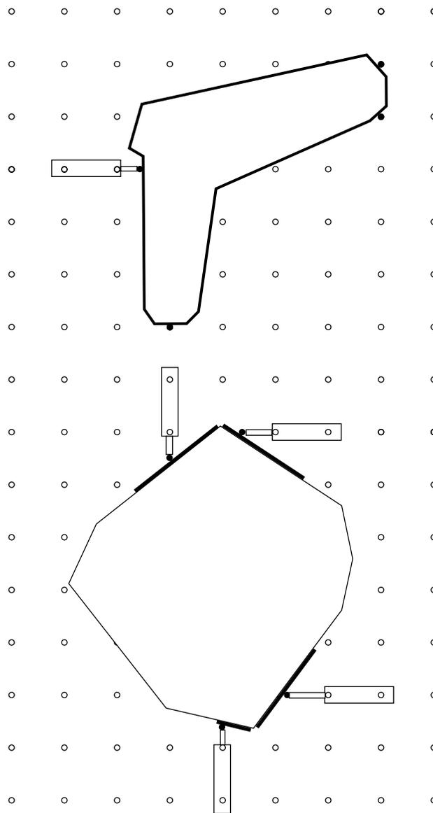
**Figure 1:** Examples of parts in modular fixtures. At top, a part fixtured with 3 locators and one clamp. At bottom, a part fixtured using 4 clamps.
