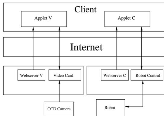
Figure 2: System architecture: each client runs two applets, Applet V for video feedback and Applet C for control.
