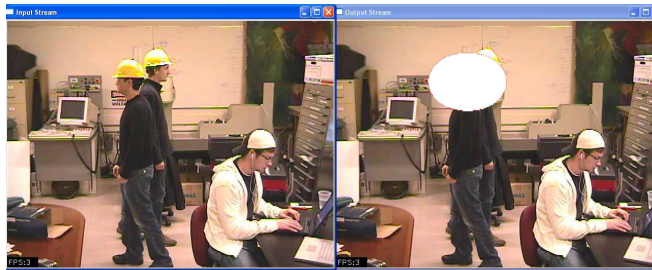
Fig. 4 Example of Crossing Markers and the Respectful Cameras System: A sample image frame input on left image, with output regions overlaid on right image. This sample illustrates tracking during a crossing, showing how the Particle Filter grows to accommodate both hats.
