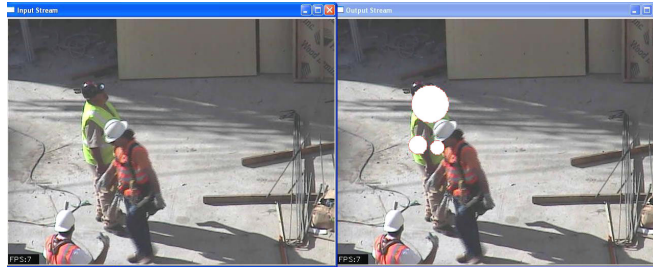
Fig. 6 Sample image frame input on left image, with output regions overlaid on right image. This sample illustrates how without Particle Filtering, even with the nine dimensional color-space, partial occlusions segment the visual marker, resulting in multiple small ellipses.
