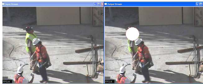
Fig. 7 Sample image frame input on left image, with output regions overlaid on right image. This sample illustrates how Particle Filtering overcomes partial occlusions, when using the nine dimensional color-space, yielding a single large ellipse.
