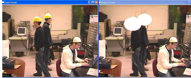
Fig. 5 Example of the Respectful Cameras System: A sample image frame input on left image, with output regions overlaid on right image. This sample illustrates tracking after a crossing (one frame after Figure 4), showing how the system successfully creates a second filter to best model the current scene.
