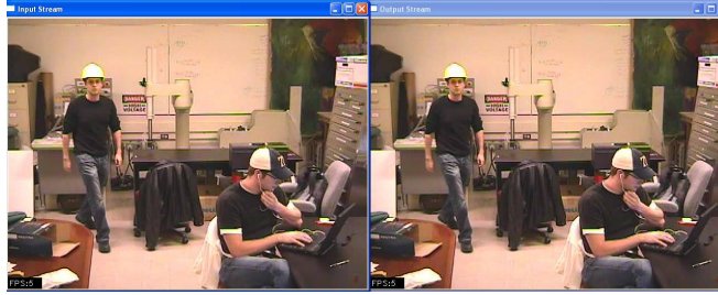
Fig. 3 Example of a False Negative with the Respectful Cameras System: A sample image frame input on left image, with output regions overlaid on right image. This sample illustrates where an intense light from a flashlight induced a specularity, causing the classifier to lose track of the hat. As a result, the right image has no solid white ellipses overlaid on the face as it should.
