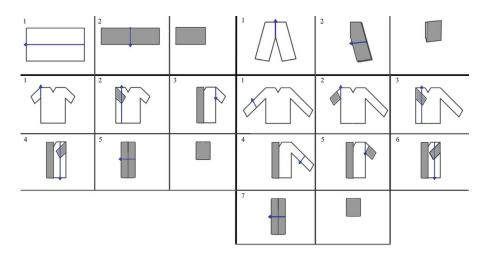
**Fig. 12.** The sequences of folds used in our experiments. Note that the long-sleeved fold is identical to the short-sleeved fold, with added folds for tucking in the sleeves. This may well be seen as a single primitive, parametrized about the sleeve length.
