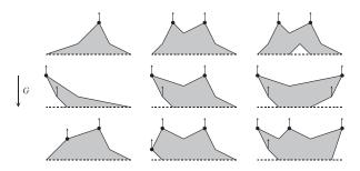
**Fig. 2.** Examples of vertical parts of cloths in various configurations. In order for the cloth not to deform, all convex vertices not at the baseline at which the negative gravity vector (small arrows) does not point into the cloth must be grasped. These vertices are indicated by the dots.
