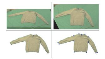
**Fig. 16.** The dataset pipeline. Top left: Initially, the clothing is spread out on a green table. Top right: A birdseye transformation is then performed. Bottom left: The image is cropped, and the background is segmented out. Bottom right: To provide ground truth for the fitting procedure, the resulting image is hand-annotated.
