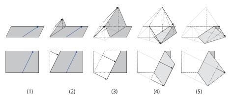
**Fig. 3.** The motion of two grippers (arrows) successfully performing the first g-fold specified in Figure 5(a) shown both in a threedimensional view and top view. At all times, all parts of the cloth are either vertical or horizontal and the cloth does not deform during the manipulation. The boundary between the vertical part and the horizontal part of the cloth is called the *baseline*.
