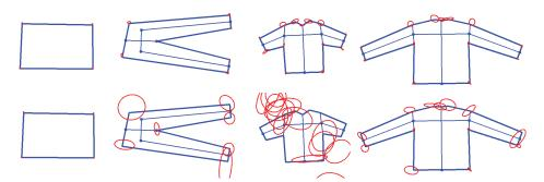
**Fig. 17.** Comparison of individual landmark point errors. The center of the ellipses denotes mean error, and the size and skew their covariance, projected onto a canonical version of the article. Top: Pointwise error for skeletal models using the PCA approach. Bottom: Pointwise error for polygon models.
