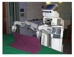
**Fig. 1.** The PR2 robotic platform (developed by Willow Garage) performing a g-fold on a towel.
