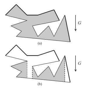
**Fig. 21.** A polygon with two upper strings shown thick. (b) The white part of the polygon (including the vertical dashed edges) has proven immobilized. The grey part remains.
