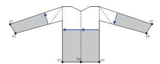
**Fig. 7.** The geometry in the long-sleeve T-shirt example after subdividing the facets by the line segment specifying the sixth g-fold. The gray facets need to be folded. The convex vertices for which the negative gravity vector points outside of the facet are shown using dots.
