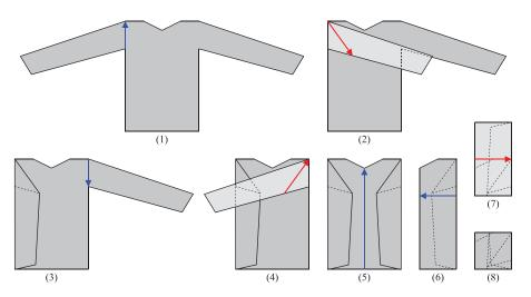
**Fig. 4.** Folding a long sleeve into a square using a sequence of seven g-folds. 'Red' g-folds apply to the geometry that was folded in the preceding g-fold. 'Blue' g-folds apply to the entire stacked geometry.
