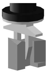
FIG 2. Computed Grip for Parallel-Jaw Gripper.
