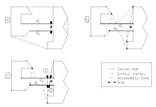
FIG 14. The steps for generating accessibility cones and modifying grips. a: Finding the convex hull of the part when a grip is inaccessible; b: Determining the critical vertices and accessibility cones; c: Creating the modified accessibility cones, and modifying the grips to [1] accessible minimum  $\phi$  grip, and [2] accessible minimum  $\delta$ ) grip.
