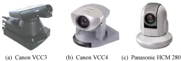
Fig. 7 The pan-tilt-zoom cameras tested with our system
