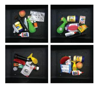
Fig. 4: Example bins from the WISDOM-Real test set. The number of objects in each bin was chosen from a Poisson distribution with mean 5, with a minimum of two objects per bin. The highly-varied geometry and occlusions make these bins challenging to segment.
