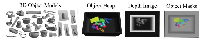
Fig. 2: Dataset generation procedure for the WISDOM synthetic dataset. A subset of 3D CAD models from a training dataset of 1,600 objects are dropped into a virtual bin using dynamic simulation with pybullet. A virtual camera captures both a synthetic depth image of the scene and object segmasks based on the pixelwise projection of each unique 3D object. This process is repeated to generate 50,000 images.
