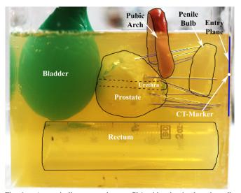
Anatomically-correct phantom Ph1 with robot-implanted needle Fig. 6. configuration A1. The organ boundaries and actual needles positions are highlighted. All sensitive structures were spared needle puncture.
