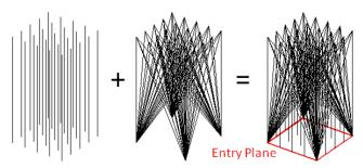
Fig. 4. The candidate needle set is the set of needles that are available during needle planning. As shown in the figure, the candidate needle set for this study consisted of: parallel lines, and skew-lines. The entry plane, which represents the bounded region on the perineum within which needles can enter the phantom is also depicted.
