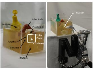
Fig. 3. Prostate phantom (5in x 5in x 8in) (left) and insertion setup (right). The anatomy modeled in the phantom includes: prostate; urethra; bladder; penile bulb; pubic arch; and rectum. A CT marker is centered on the square entry zone for calibration. As shown in the right image, the Acubot-RND is registered to the CT-marker.
