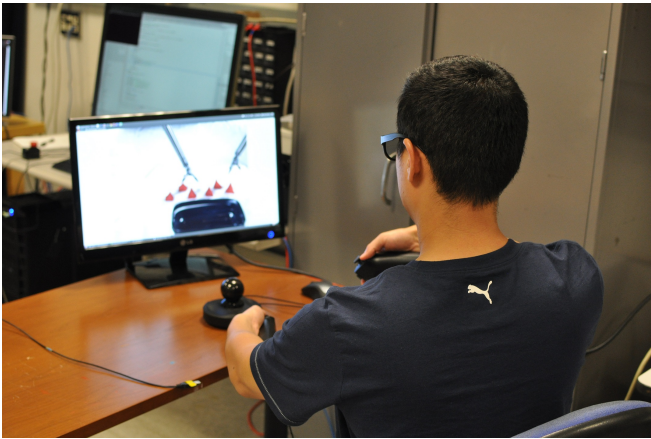
Fig. 5. Setup for human local teleoperation, using a 3D monitor and the Razer Hydra controller.
