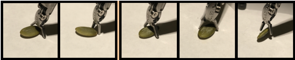
Fig. 8: Properties of pumpkin seeds during debriement. These seeds slide and rotate on the paper surface. Type A errors frequently result in the seed getting pushed out of the gripper’s control (first two images). This can also happen even if calibration is accurate and the dVRK ends up in a reasonable location. The third image shows a gripper initially in an excellent spot to grab the seed, but one tip can rotate the seed before it gets gripped (fourth image) which can cause it to snap out of control (fifth image). This is a type B error.
