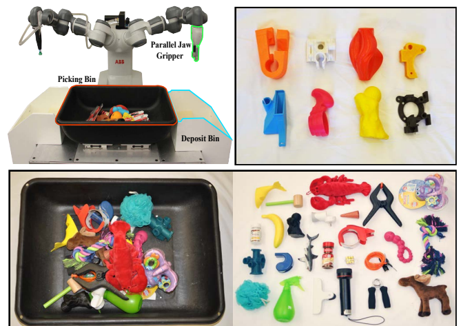
Fig. 3: (Top Left) The experimental setup consisting of an ABB YuMi with custom silicone fingertips [7] and a high-res Photoneo PhoXi depth sensor. The experimental objective is to move objects from the picking bin to the deposit bin. (Top Right) The 8 adversarial objects used by Mahler et al. [21]. (Bottom Right) The 25 novel objects with diverse geometries used to test generalization. (Bottom Left) The 25 novel objects arranged in a bin to simulate dense clutter.
